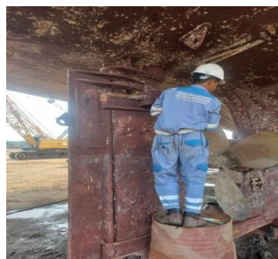
Gambar 3.1 11 pengukuran as kemudi
