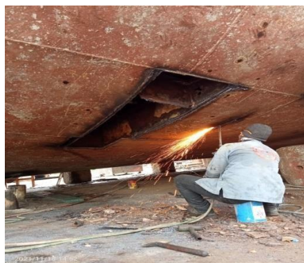
Gambar 2 13 gambar proses replating Roro KMP. Swarna darma
