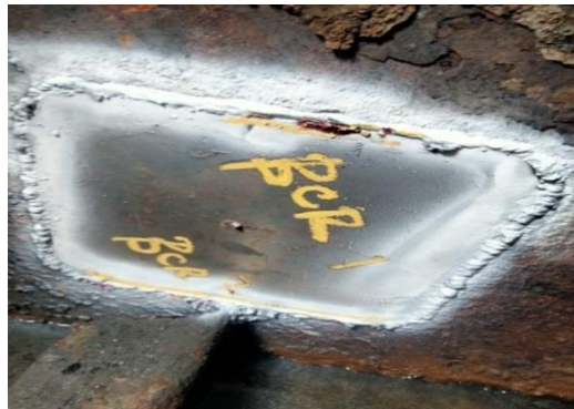
Gambar 2 6 Proses penetrant Test kapal artha
