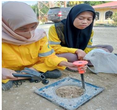
Gambar 3. 20 *Send Cone Test*
