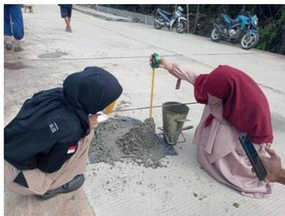
Gambar 3. 8 *Slump Test*
