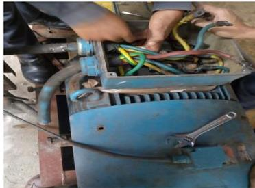
Gambar 2. 12 Connect Elektro Motor Bd6
