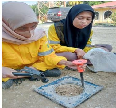
*Gambar 3. 18 Send Cone Test
