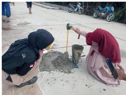
Gambar 3. 7 *Slump Test*
