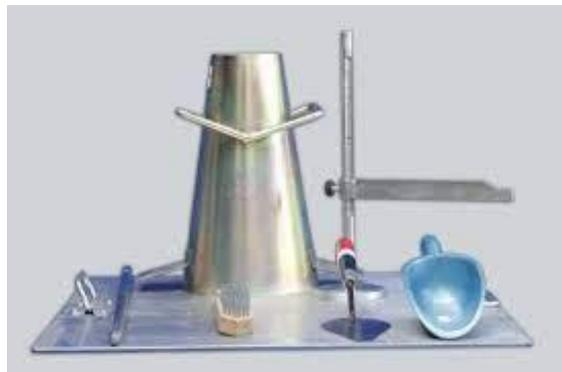
Gambar 3. 20 Alat slump test
