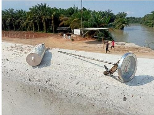
Gambar 3. 19 Thermometer aspal
