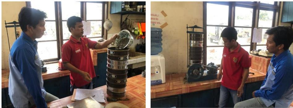
Gambar 4. 8 Pengujian material properties/gradation
