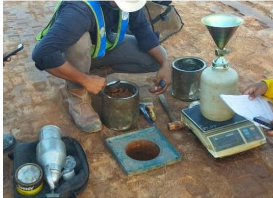
Gambar 3. 25 Sand cone test
