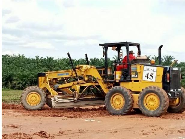
Gambar 3. 5 Motor Grader
