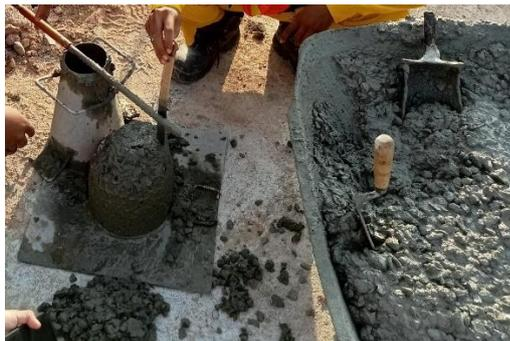
Gambar 3. 42 Uji Slump Beton
