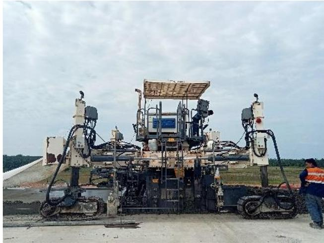
Gambar 3. 11 Concrete Paver
