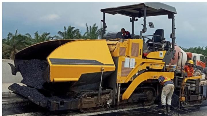
Gambar 4. 2 Asphalt paver
