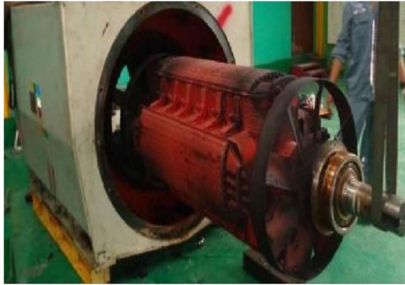
Gambar 4. 4 Proses Pembongkaran Rotor (Sumber: Laporan Report Incoming Inspection PT. IndoTurbine)
