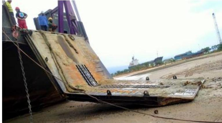
Gambar 1. 1Kondisi Ramp Door Mengalami Patah
