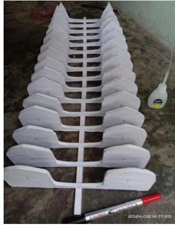
Gambar 4.13 Proses Fit-Up setiap stasion
