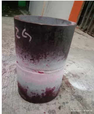
Gambar 4.75 Hasil Penetrant test Butt Joint 2G Sumber: Penulis
