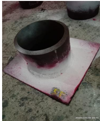
Gambar 4.74 Hasil Penetrant test Tee joint 5F Sumber: Penulis
