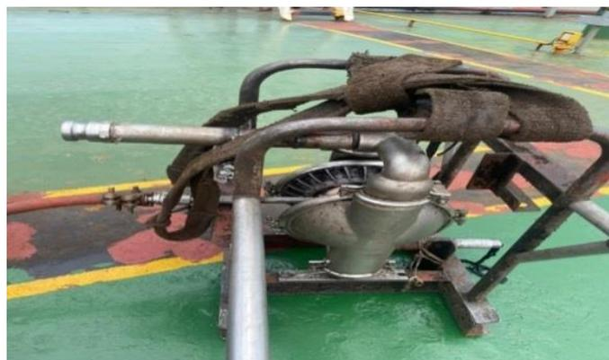
*Gambar 3.2 Alat Pompa Tangki (Cargo Pump)*
