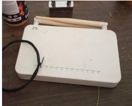
Gambar 3.2 3 Optical Network Terminal
