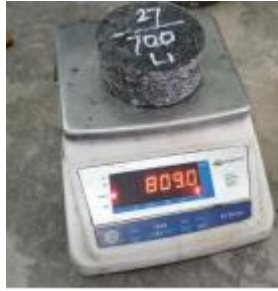
gambar 3. 11 Timbang kering sampel core drill
