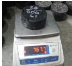
gambar 3. 14 Menimbang berat sampel core drill berat SSD
