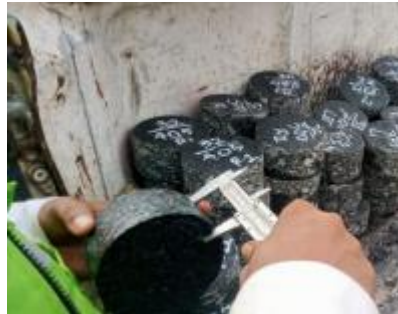
gambar 4. 10 Pengukuran Ketebalan Hasil Core Drill
