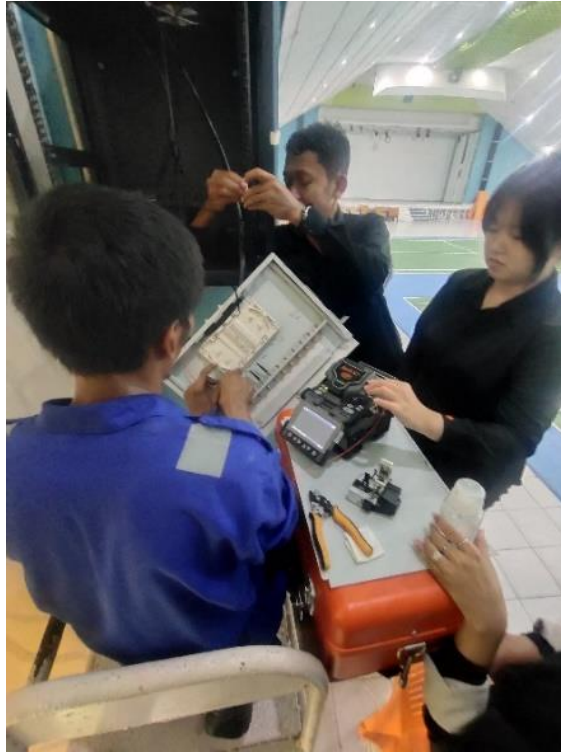
Gambar 3. 4 Terminasi Fiber Optic
