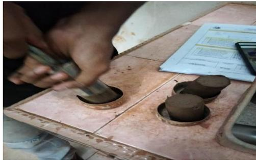
**Gambar 3.24** Pengujian Kadar Air Dan Berat Volume
