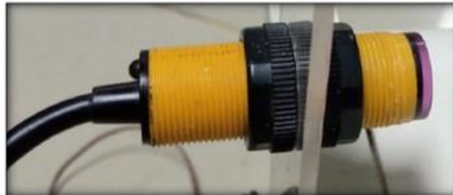
Gambar 2.8 Sensor Proximity D18-3430P1 Sumber: (Wahyudi, 2020)
