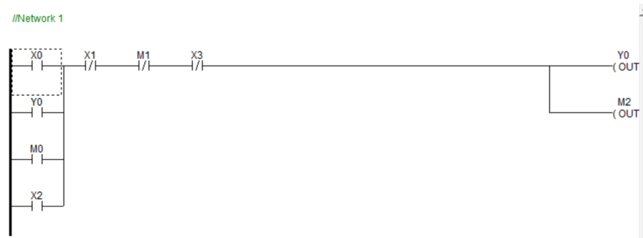
Gambar 4.5 Ladder Software PLC Praktikum 2 Sumber: (Dokumentasi, 2024)
