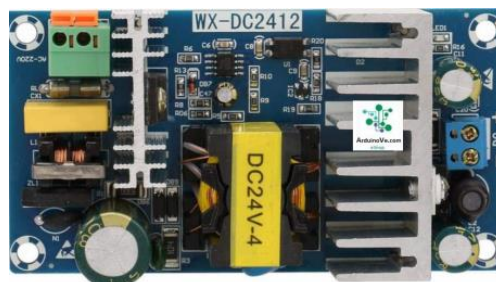
Gambar 2.15 Power Supply WX-DC2412 Sumber: (Rahman, 2023)
