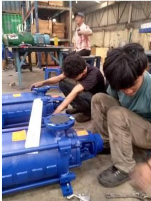
Gambar 1 Disassembly Pompa Multistage
