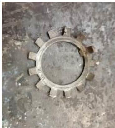
**Gambar 4. 15 Gambar Lock Washer**
