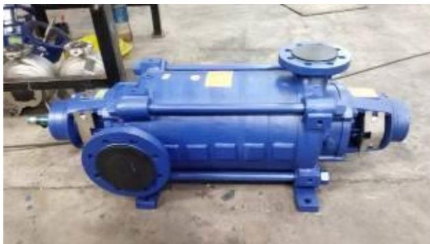
**Gambar 4. 1 Pompa Multistage D65**
