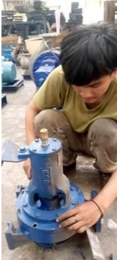
Gambar 3. Assembly Pompa Ethanom
