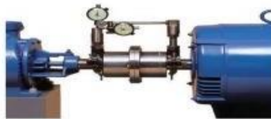
Gambar 4. 2 Metode Alignment Dial Indicator (Sumber : Suker junior,2022)
