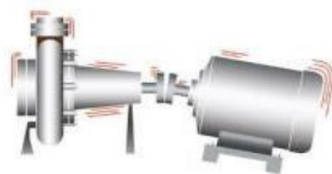
Gambar 4. 5 Ilustrasi Missalignment (Sumber: maintworld.com)
