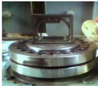
Gambar 4. 3 metode Alignment level precision (Sumber : Suker junior,2022)
