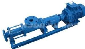
**Gambar 4.8** pompa screw
