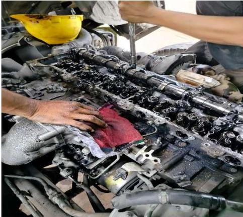
*Reaseal cover silinder head replace water pump loader 02 NPP HDD air coolant*
