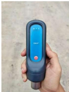
**Gambar 4.13** Vibrasi Pen SKF CMDT 391
