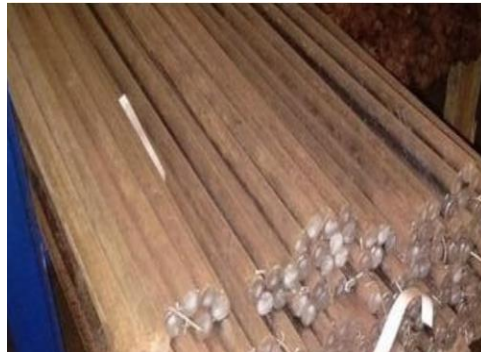
Gambar 4.1 As Chaingrate (as pin) Sumber: Dokumentasi Pribadi
