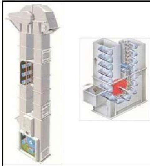
**Gambar 4. 1** *3D Elevator Chain*
