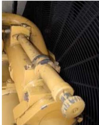
Gambar 4.8 Fuel Priming Pump
