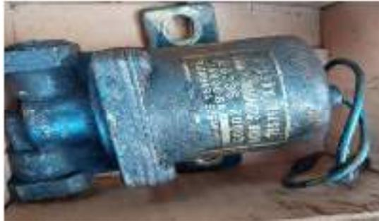
Gambar 4.9 *anomometer switch*( switch angin)
