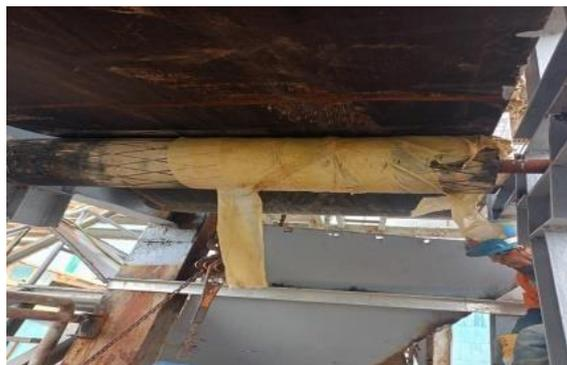
Gambar 4.6. *Model Snubb Pulley*
