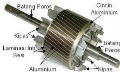
Gambar 4. 3 Rotor
