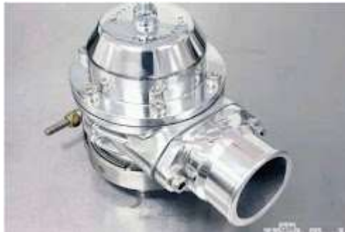
Gambar 4.26 Blow off Valve
