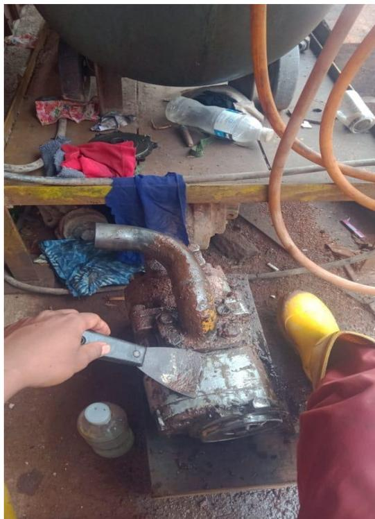
Gambar 4. 5 Pompa Hidraulik Wheelloader
