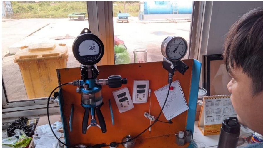
Gambar 2. 12 Calibration pressure gauge di lab calibration (Sumber: Dokumentasi, 2024)
