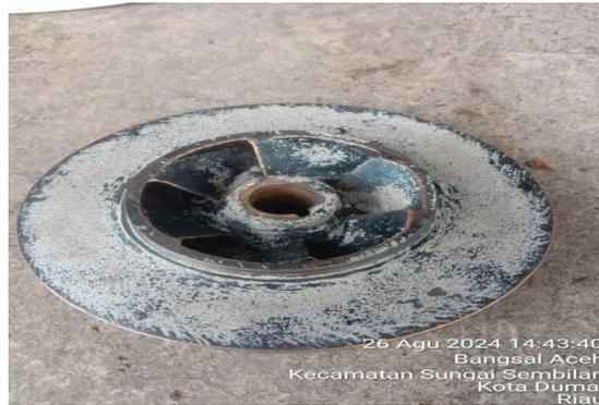
Gambar 4.6 Impeller
