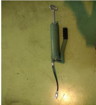
Gambar 3. 19 Grease pump
