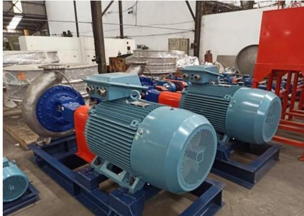
Gambar 4. 1 Pompa Sentrifugal
