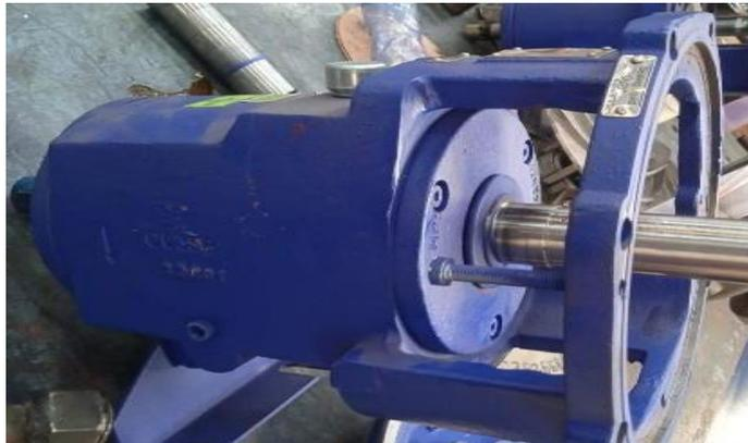
Gambar 4. 7 Bearing Housing
