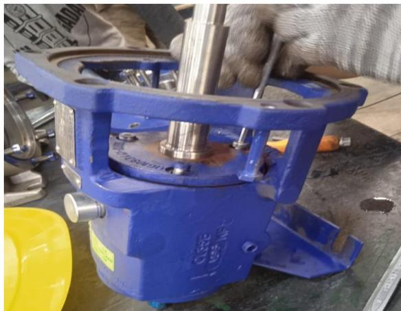
Gambar 4. 15 Memasang bearing cover pada bearing housing
