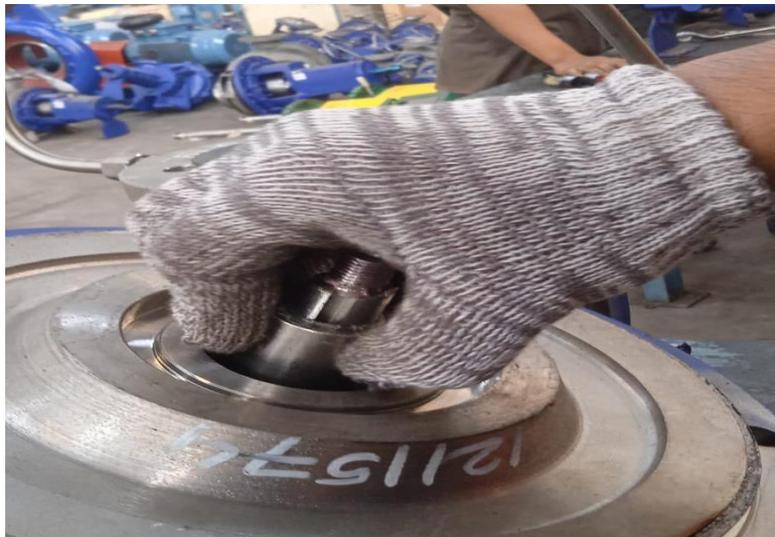
Gambar 4. 18 pemasangan mechanical seal
