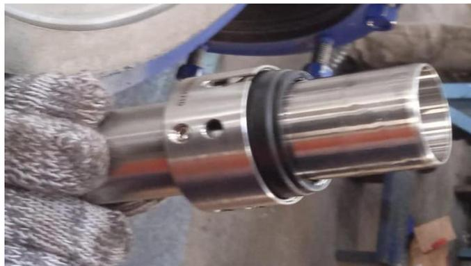
Gambar 4. 9 Mechanical seal
