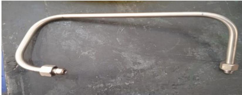
Gambar 4. 12 Pipa *flashing*
