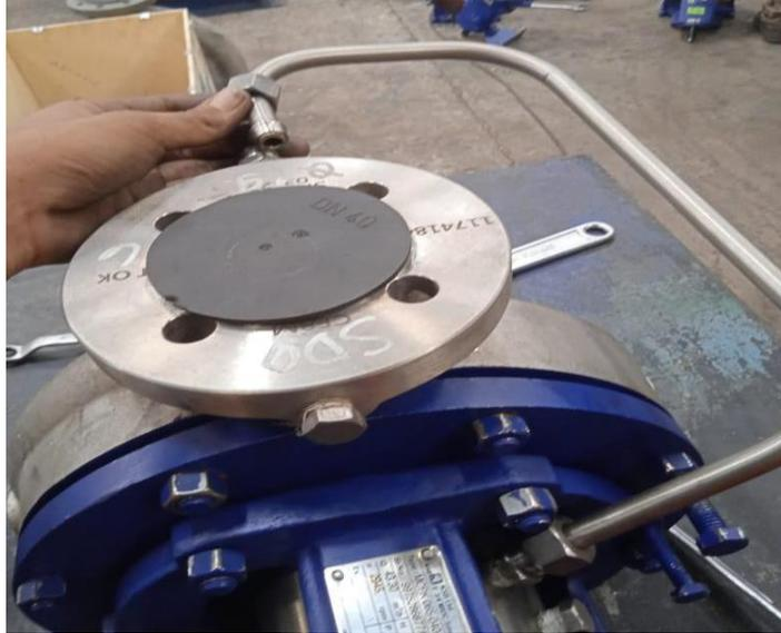
Gambar 4. 21 Pemasangan pipa flashing
