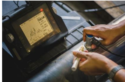
Gambar 4. 15 Phased Array Ultrasonic Testing
