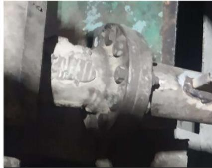
Gambar 4. 20 *Coupling Shaft*
