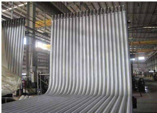
Gambar 4. 8 *Wall tube Boiler*
