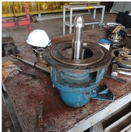
Gambar 4. 13 Finishing pemasangan Bearing
