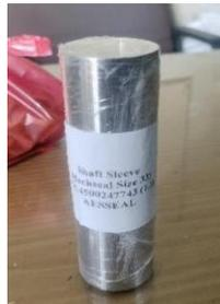
Gambar 4. 17 *shaft sleeve* baru
