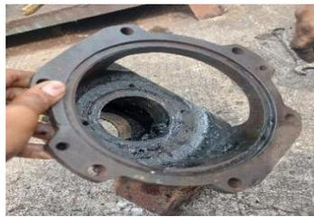
Gambar 4. 12 *Bearing Housing*
