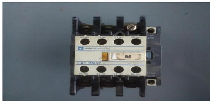
Gambar 3.7 *contactor (Magnetic Contactor)*
