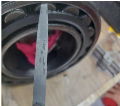
**Gambar 4. 19 Clearance Bearing Longgar**
