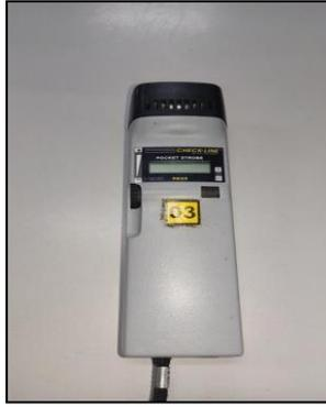
**Gambar 3. 1 Stroboscope**
