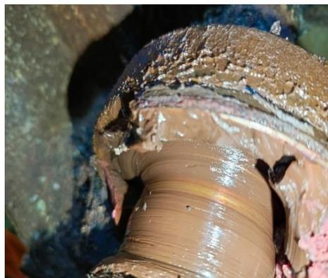
**Gambar 4. 20 Bearing contamination**
