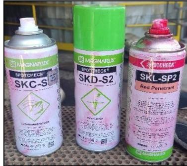
**Gambar 3. 8 Liquid Penetrant Test**
