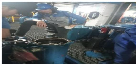
**Gambar 2. 22 Reaplace filter booster**
