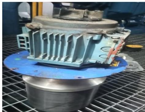
*Gambar 4. 11 motor oil mist separator
