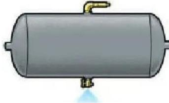
Gambar 4.4 Air Reservoir Tank
