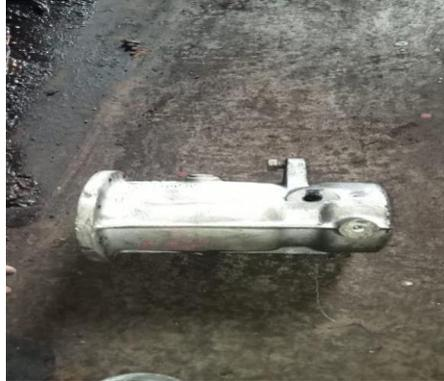
Gambar 1 9 housing bearing
