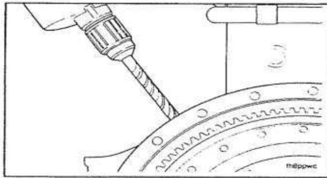
2. Bor lubang berukuran 3/16 inci 147 mm dihousing.
