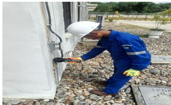
**Gambar 2. 6 Pengukuran Grounding**
