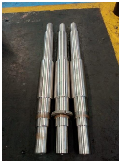
Gambar 4.15 Shaft Pump Rejeck Centry Filter PM-8
