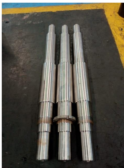
Gambar 4.15 Shaft Pump Rejeck Centry Filter PM-8
