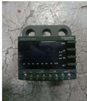
Gambar 3.3 Electronic Over Current Relay (EOCR) (Sumber: Dokumentasi, 2024)
