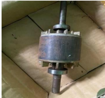
Gambar 3.2.1 rotor blower motor 1 phasa (Sumber:Unit Pertamina Sei Pakning 2024)
