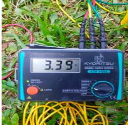
Gambar 3.3 Alat ukur grounding (Earth tester) (Sumber: Dokumentasi Penulis,2024)
