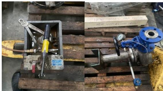
*Gambar 4 15 Alat Presser Test*
