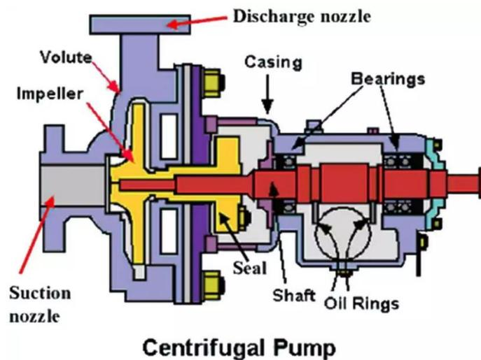
*Gambar 4 1 Pompa Sentrifugal*
