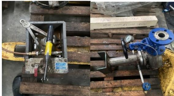
*Gambar 4 15 Alat Presser Test*
