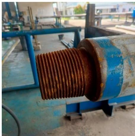
Gambar 4. 1 *Heavy weight drill pipe*
