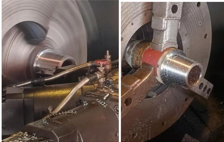
**Gambar 4. 6 Proses *Threading***
