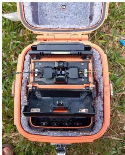
*Gambar 4. 3 Proses Splicing*
